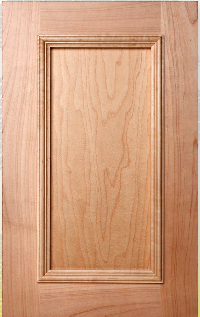
5-PIECE DRAWER FRONT Minimum Height: 6" with 1-1/2" Rails
